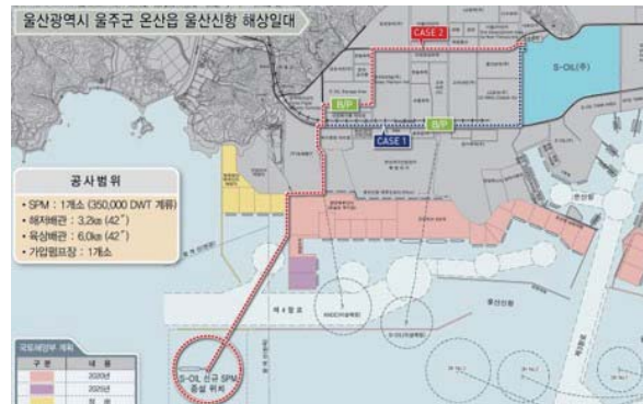
S-OIL New SPM and Pipeline Project (Korea) Basic & Detail ENG-42"-7km Submarine Pipeline and PLEM, SPM Refurbish, Detail Engineering
