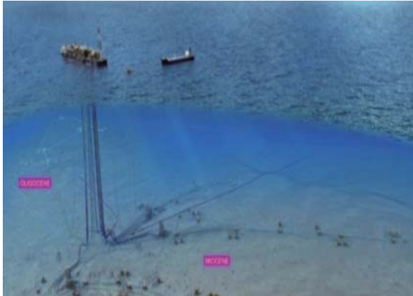
JAZAN Refinery and Marine Terminal Project (Saudi) Detail Engineering for Offshore Pipeline 2-Lines 48"-8km and PLEM/SPM & 2ND SPM (2-Line x 2.5km)
