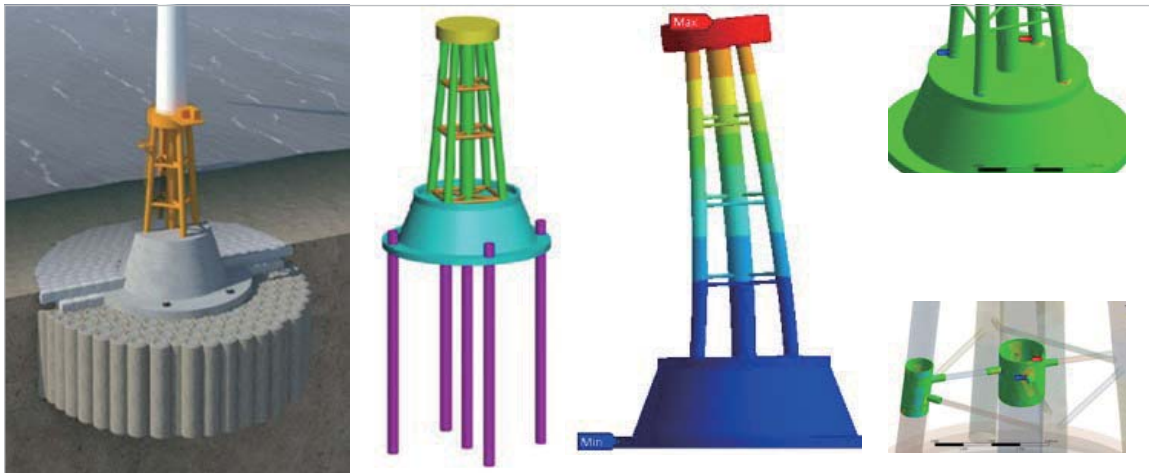
Development of Hybrid Substructure Systems for Offshore Wind Power, Korea Evaluation Institute of Industrial Technology (KEIT) - Design of hybrid type substructure of offshore wind power to improve structural performance
